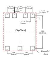
\* Do not route any traces in the keep out area. It is recommended the next layer under the keep out area is to be ground plane.
