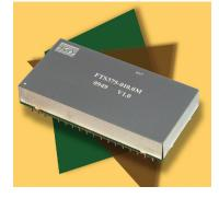
MHz SINE output from an intrinsically low jitter voltage controlled crystal oscillator. The FTS375 can lock to a 10 MHz reference derived from the on-board GPS receiver or an external 10 MHz reference or to an external 1 PPS reference. Alarms are provided to indicate Loss-of-Lock, Holdover, and Antenna Fault. The on-board GPS receiver requires an outdoor mounted GPS antenna for the best stability and consistent performance.
