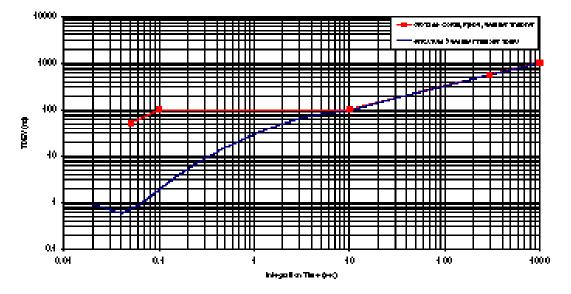
The SM3, when configured for the appropriate stratum 3 bandwidth frequency, meets the stratum 3 requirements, **Jitter Generation** – Jitter generation is the process whereby jitter appears at the output of a clock in the absence of input jitter. The device jitter generation performance is as shown below:
