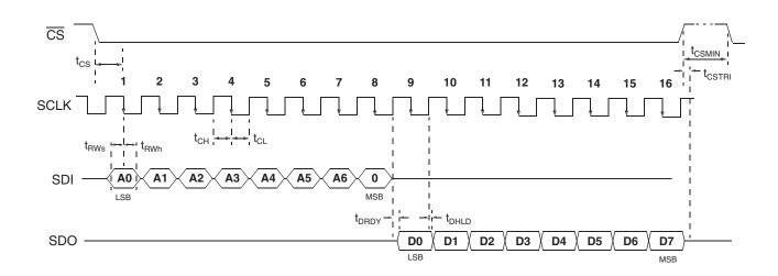
**Serial Interface Timing, Write Access**
