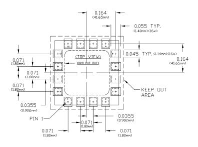
KEEP OUT AREA UNDER THE PCBOARD IS A KEEP OUT AREA, DO NOT PLACE ANY PARTS IN THIS AREA.
