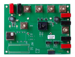
the FT9-P series, the MCLK\_IN BNC connector at J4 is used as the REF\_IN for the -P series modules, not the REFIN\_1 and REFIN\_2 connectors at J11 and J12.
