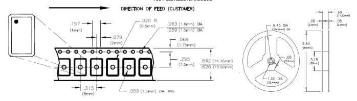
Tape and Reel Information for Alternate T-series package outline models T602-010.0M, T602-019.2M, T602-020.0M, and T602-030.72M Meets EIA-481A and EIAJ-1009B 1000 PCS/Reel Maximum
