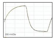
Note: The clipped sinewave output is AC coupled
